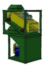
The SD600DP Primary Shaker is a high capacity, declined, single deck shaker with 2 No. discharge pumps, used for the separation of coarse particles or clay balls. The SD600DP consists of a shaker module, which mounts on top of a pump tank module. These two units wedge together to form an ISO Type 1CC 20 foot ISO container sized unit for transport. The machine also includes a free-standing Metso pump which is transported separately.
