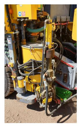
${\color{red} \textbf{Comments:}} \ \, \textbf{Crout boom is in good working condition rig has 3/4} \\ \text{bulbed cable still fitted and grout hose is in good condition, Cable cutters} \\ \text{and drive motors have no leaks}$
