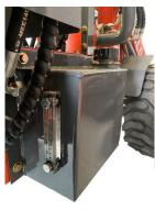
The hydraulic system is topped up from the cap adjacent to the accelerator pedal. The hydraulic tank capacity is 11 litres and should be inspected regulary. A site gauge sits at the rear of the tank.
