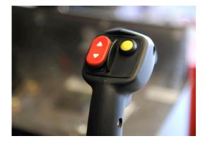
Upward arrow is selected to drive forward. Central position is neutral.
