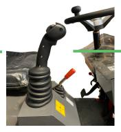
Push the joystick forward to lower the lifting arm and the attachment.
