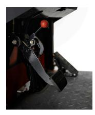
The accelerator pedal is on the right and the brake is on the left hand side of the footwell. The brake also has a manual park brake, controlled by the red handle.
