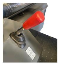
Brumby uses a Quick Hitch system to connect attachments. Attachment must be in an on-ground safe position before using the quick hitch control leaver. Forward movement on the quick hitch handle will release the locking pins to enable removal of the attachment. Always return the quick hitch leaver to its locked position. The hydraulic three way valve leaver needs to be in the Quickhitch position. CAUTION - always ensure the locking pins are correctly in place before using any attachment.
