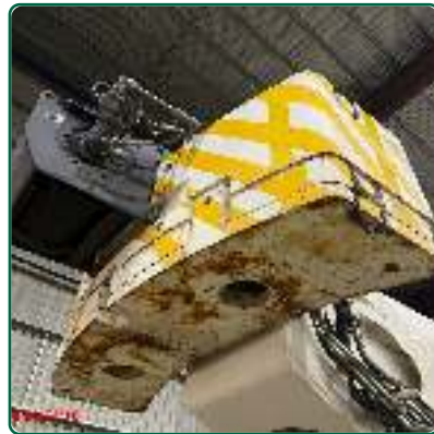
Counterweight Hazard Striping
