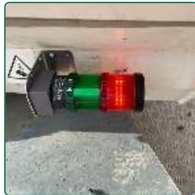
Overload Warning Lights and Alarms
