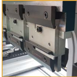
Reversible punch-holders with manual quick clamp
