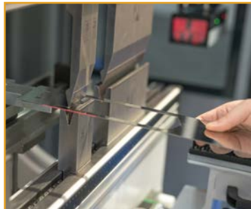
IRIS PLUS: angle measurement system (integration only with Adcontrol 60)
