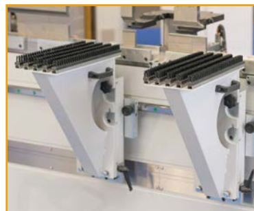
Front support arms on rail (with brushes and height adjustment)
