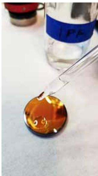
*Figure 7-12. Methanol on Lens*
