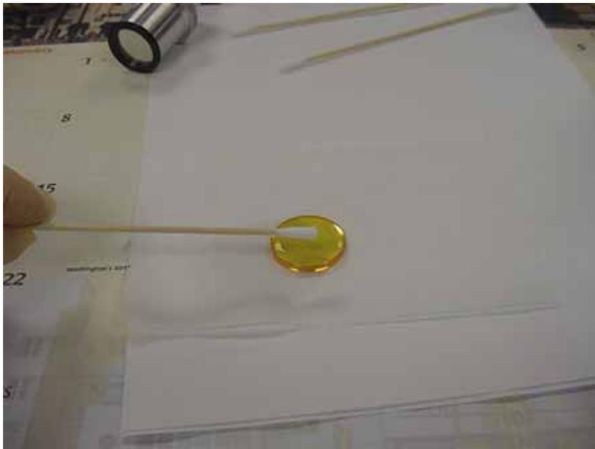
***Figure 6-8. Optic Window Cleaning with Swab***
