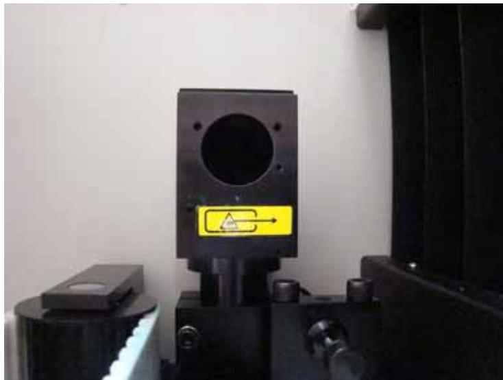
Radiation Exposure Warning Label on Beam Bending Mirror
