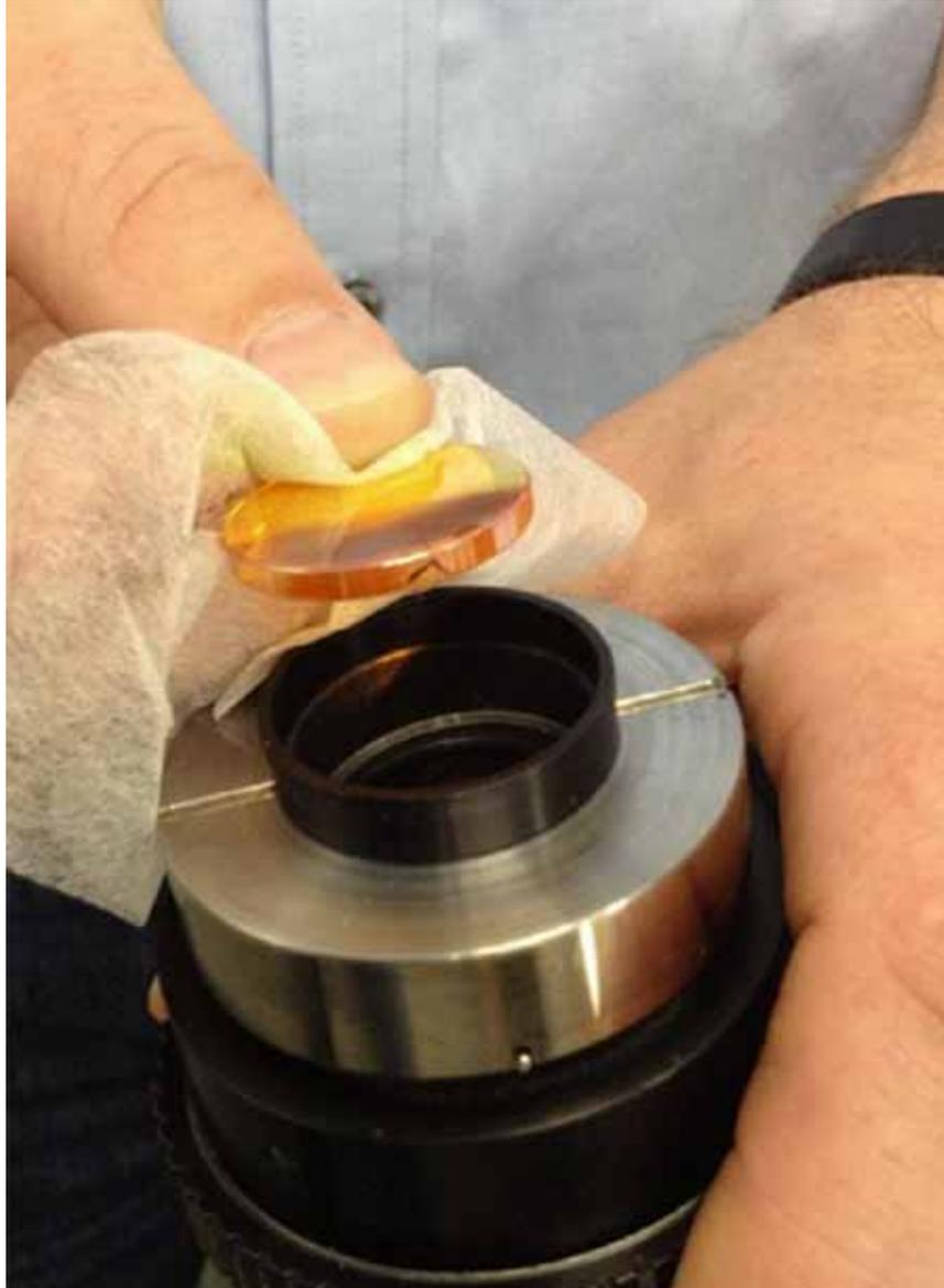
***Figure 6-10. Installing the Optic Window***
