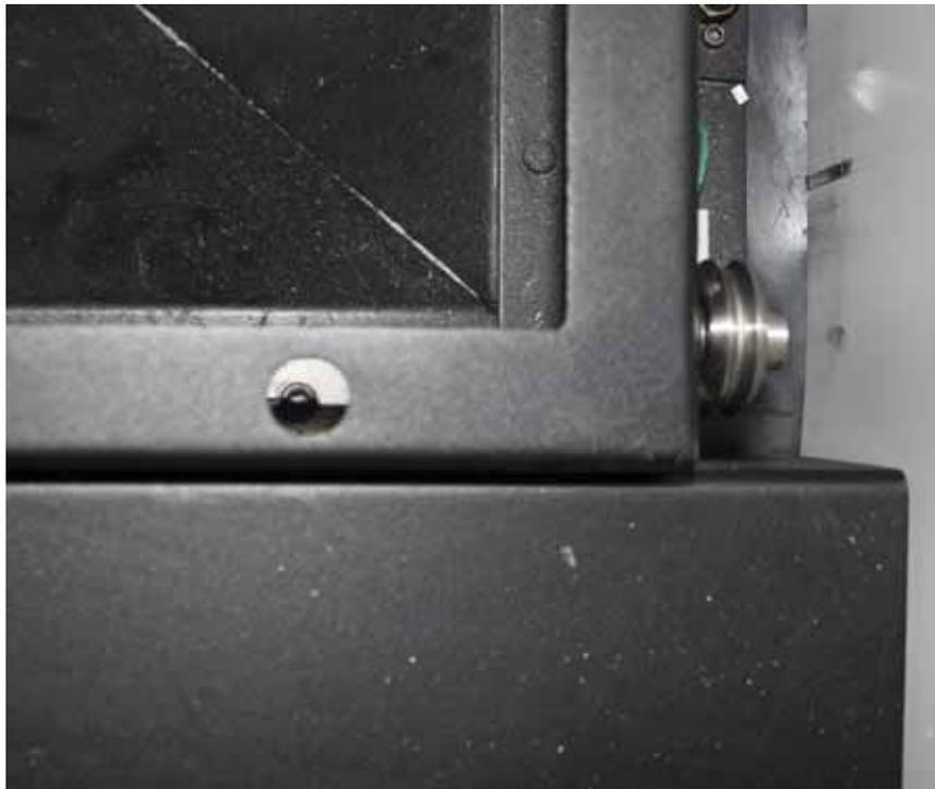
***Figure 6-15. Cutting Bed Corner Adjustment Screw***
