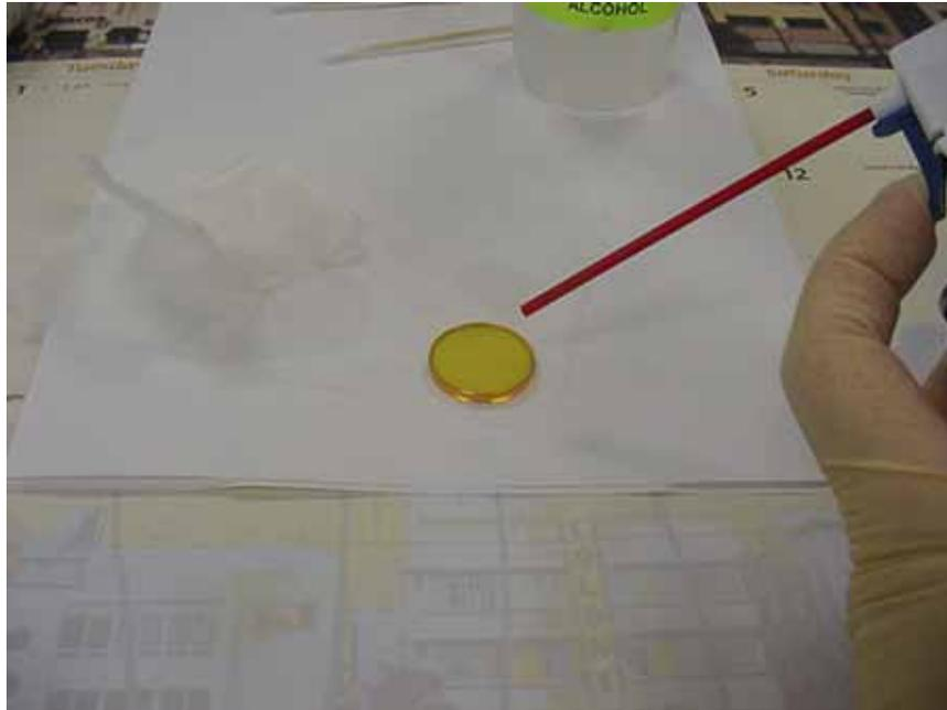
**Figure 6-9. Optic Window Cleaning with Canned Air**
