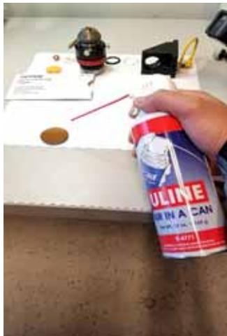
*Figure 7-11. Clean with Compressed Air*
