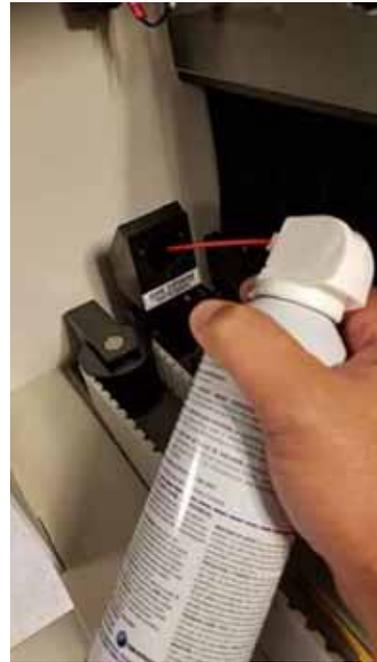
***Figure 7-6. Use Compressed Air to Clean Off Debris***
