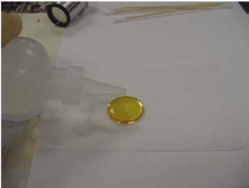
**Figure 6-6. Optic Window Cleaning with Alcohol**
