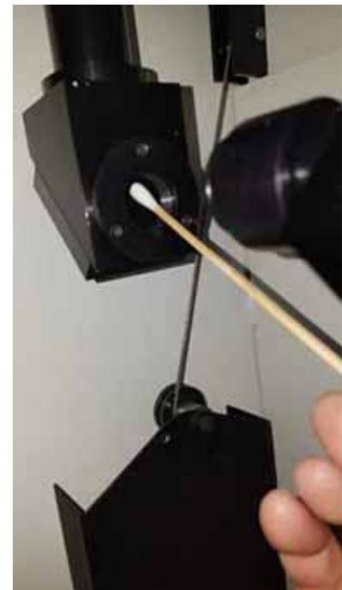
***Figure 7-7. Use Isopropyl Alcohol on Swab***
