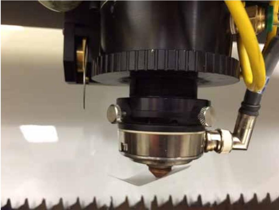
***Figure 6-16. Nozzle With Tape***
