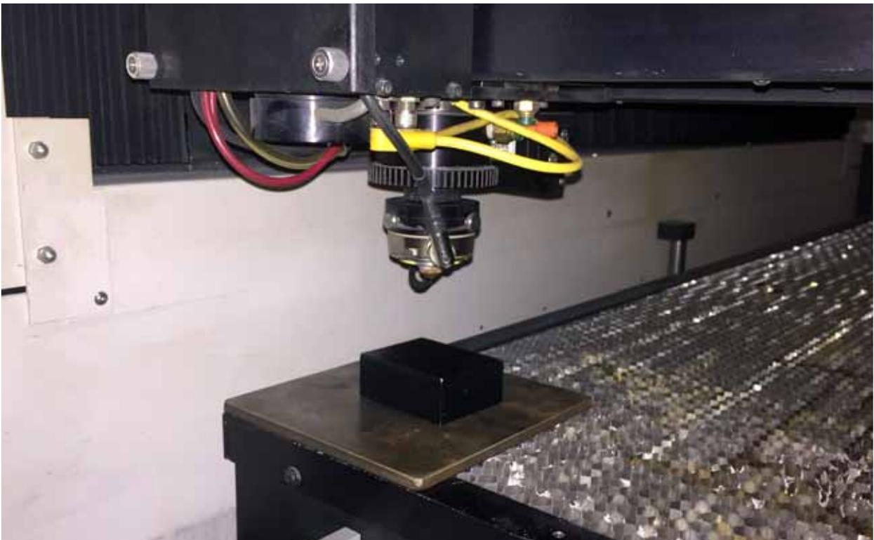
*Figure 6-14. Leveling Block*
